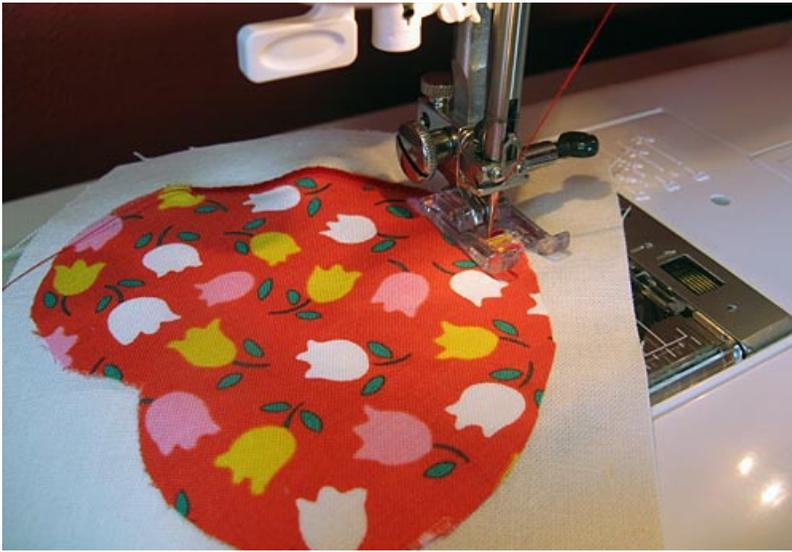
6. Don't be afraid to stop, with your needle in the down position, and adjust your fabric as you move around the curves.
