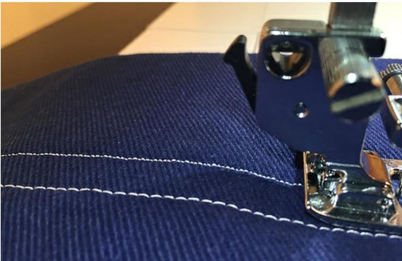
When you adjust the stitch length, it's not the needle that is changing, it's the feed dogs (those little grippers in the center of the needle plate below the presser foot). The machine alters how much fabric the feed dogs will move before making the next stitch.
