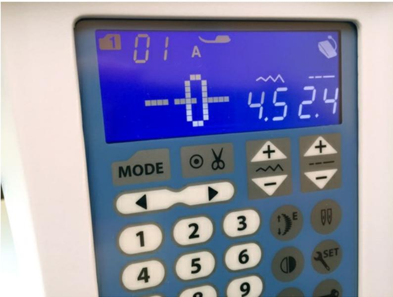
That said, you can adjust the length to best fit your situation, fabric or technique. The most common stitch length range is from 0.0 to 5.0, with 5.0 being the setting for machine basting or gathering and 0.0 the option for free-motion quilting with the feed dogs lowered. In the photo below, you can see our three lines of test stitching, from bottom to top: 5.0, 2.4, 1.0,
