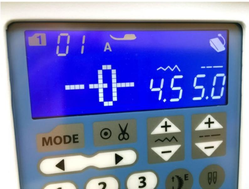
If your machine has a smaller LED screen, there may simply be an indicator light to one side of the screen, such as on the Janome Magnolia shown below. When this light is next to the stitch length symbol (often a dashed line) you can use the plus and minus buttons to increase or decrease the stitch length.
