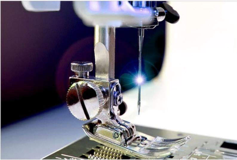
Shorten the stitch and that reduces the amount of fabric fed under the presser foot before the needle comes down. Lengthen the stitch and the feed dogs increase the amount of fabric moved under the presser foot before the needle plunges in again.
