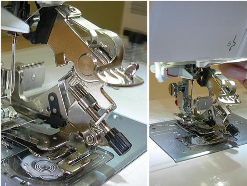
7. Select a straight stitch, and test your needle drop to make sure it goes in and out of the needle hole in the ruffler easily. There are adjusting screws on the ruffler to move the opening to best match your needle drop.
