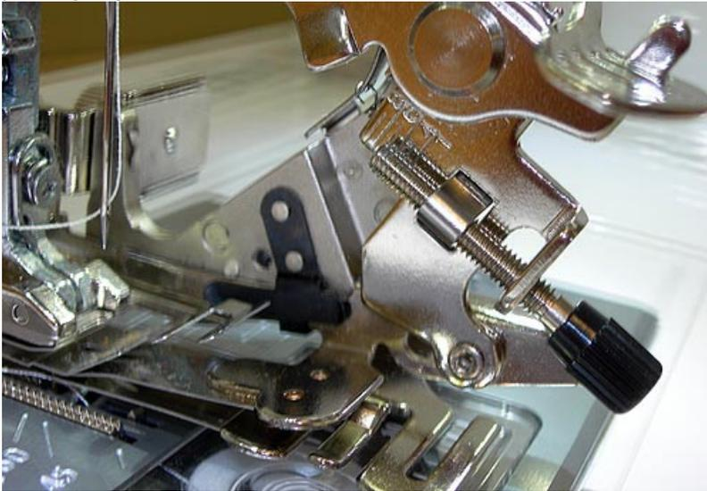
10. Insert the raw edges of your folded strip into the slit at the front of the ruffler. We started with the 1 slot for a ruffle every stitch and with the depth at about 4.
