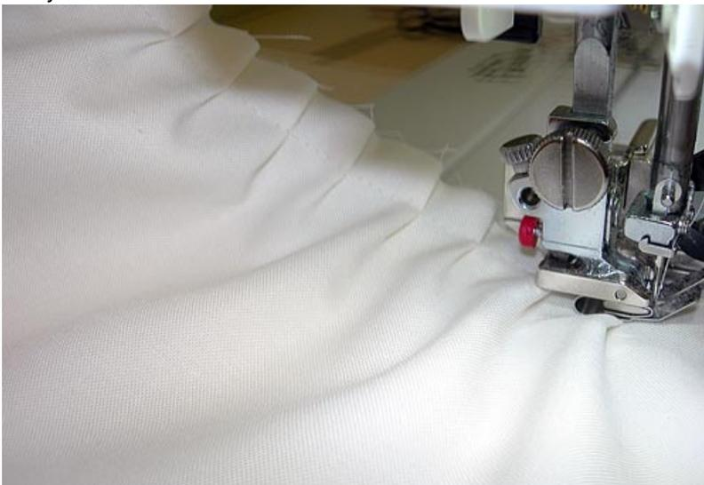
15. Then, we moved the plate into the '12 slot' and tightened the depth screw a bit more to create pleats every twelve stitches.
