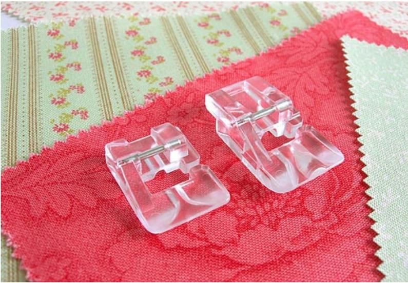
Simply remove your existing presser foot and snap on one of the two Beading feet. This foot set is manufactured by Janome for Janome machines, but may work on other models that accept snap-on feet. Check with your local dealer to be sure. Your sewing machine brand may have its own version of this type of foot.
