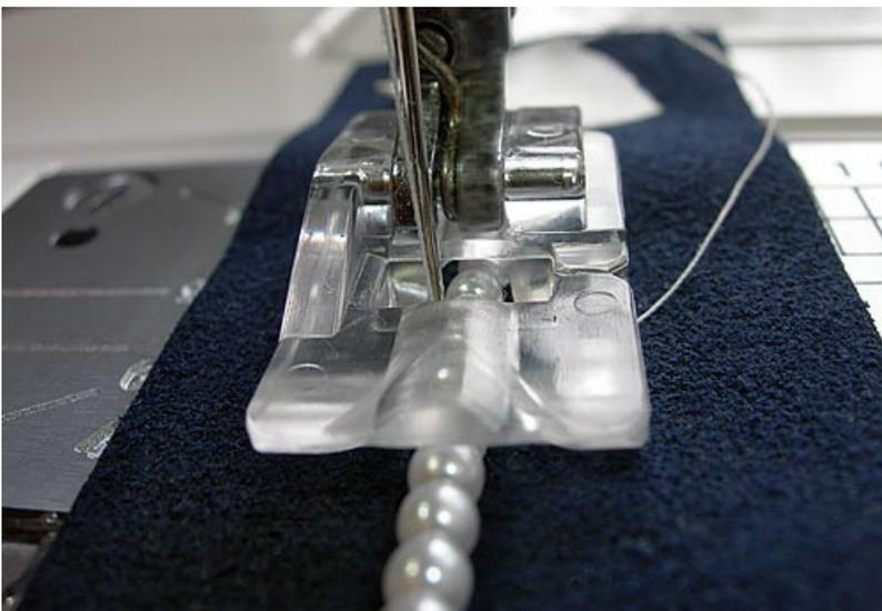
In the background of the photo above is a blurry white square we'd like to bring to your attention. Not because it's blurry, but because that is a piece of tape. Our personal hint is to use an overlapped piece of tape to 1) secure the ends of your strand so the beads don't slide off, and 2) to attach the end of the stand to your fabric.
